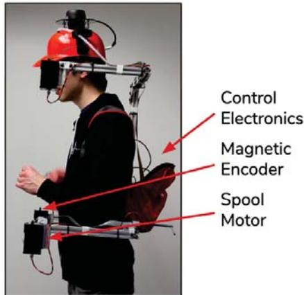
Figure 5: Electronics subsystems in context.
