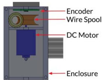
Figure 4: Schematic of one of In-Sight's three wire spools.
